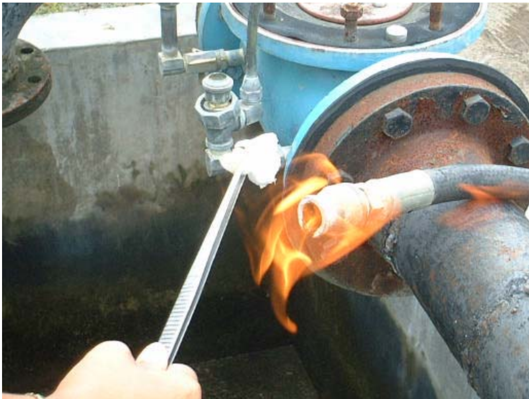
Flame cleaning of sampling port prior to sample collection
