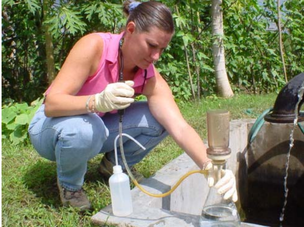
Field filtering of water samples to be analyzed for dissolved iron and manganese
